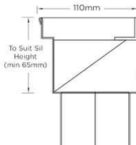
Grates longer than 1500mm supplied in sections. Tile Inserts longer than 1200mm supplied in sections. Channels over 3000mm supplied in sections with joiner. +/-2mm tolerance on dimensions.
